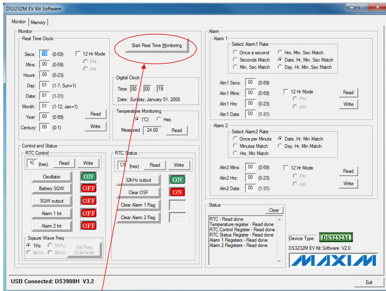
Depressing the 'Start Real Time Monitoring' button puts the application into a continuous-read loop, updating the real-time, alarm, status, control, and temperature sensor register contents. Once started, this button renames itself to 'Stop Real Time Monitoring', and the green LED (D2) on the DS3900H2 will blink red upon each component read.
